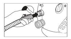
→ STEP 2: Insert the spray wand to the trigger gun. Press in against the spring tension and twist into locked position.
